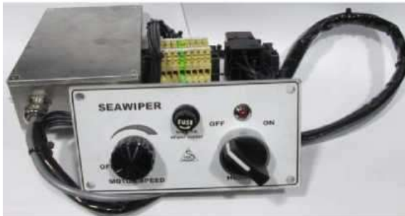
24VDC control panel for 24VDC motor and 24V heating.
