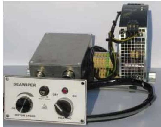
230AC/DC control panel for 24VDC motor and 220V heating.
